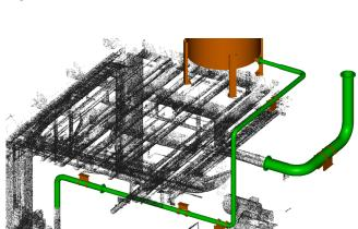
The designer can use point cloud directly when planning the pipeline route or replace the point cloud pipe with a real pipe.
