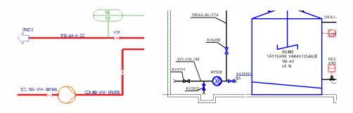
The identifiers (ID) of equipment, pumps, valves, lines etc. are dynamically placed in the diagram by pointing to the desired place with the cursor. The identifier can be freely modified as needed. The format of the ID is defined in the settings file for each project.
